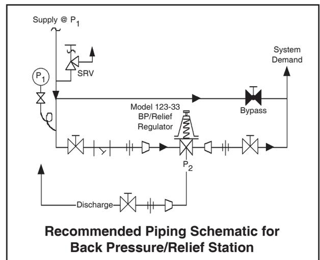
6. Clean the piping of all foreign material including chips, welding scale, oil, grease and dirt before installing the valve. Strainers are recommended.
