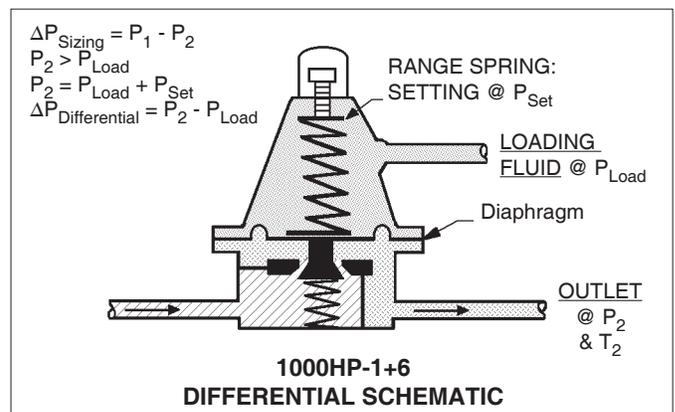
6. For a 1000HP-1+6 (single diaphragm) design, a complete diaphragm failure will cause the fluids to mix in the spring chamber or loading pressure piping system.
