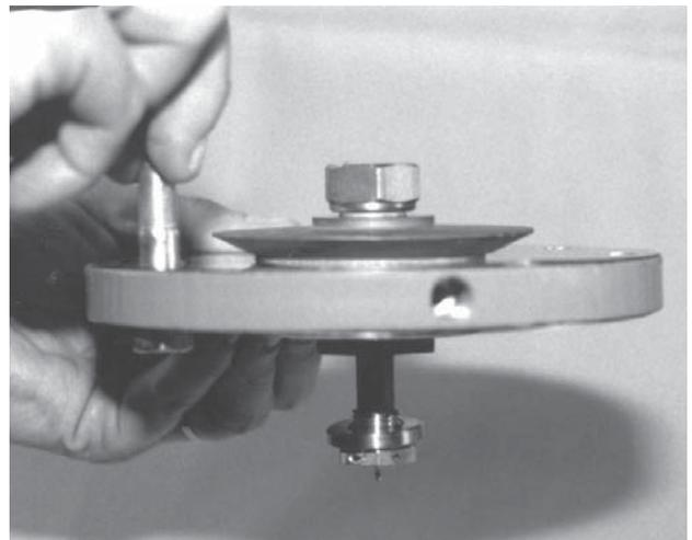
8. Remove diaphragm subassembly by sliding the pusher plate and stud (13), body spacer (42) and nut (11) in the direction of the regulator inlet, approximately 1/2"–3/4" (15-20 mm). The pusher plate and stud (13), stud nut (10), and stud collar (16) should disengage with the rocker arm (14) slot. Lift vertically for diaphragm subassembly removal, carefully holding the assembly at its outer edge to prevent the body spacer (42) from falling from between the diaphragm(s) (20).
